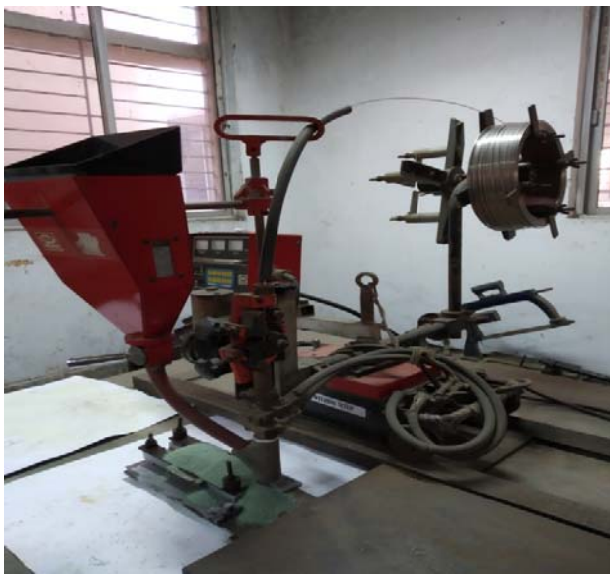
Figure 2: Submerged Arc Welding machine setup.
